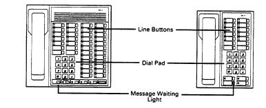
Figure 1A: Typical Merlin telephones.
